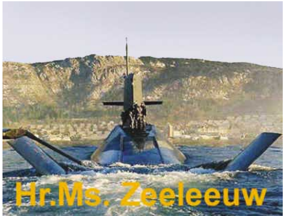
Figura 11 – Submarino Hr.Ms. Zeeleeuw (classe Walrus) – LLHH-AR em forma de \mathbf{X}
