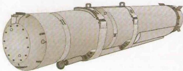
Mark 60 Captor mine. The long capsule contains sensors and a Mark 46 ASW torpedo. JACK RYAN ENTERPRISES, LTD.
