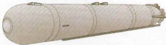
Mark 67 submarine-launched mobile mine (SLMM). This is a converted Mk 37 torpedo designed to be fired from a distance, then to sink to the ocean floor to act as a bottom mine. JACK RYAN ENTERPRISES, LTD.
