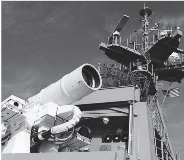
Laser Weapon System (LaWS) a bordo do USS Ponce (Foto: U.S. Navy)
