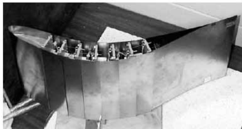
Figura 7 – Estruturas flexíveis de SMAs multiatuadas – (a) Aircraft Maneuverability (webdocs.cs.ualberta.ca/~database/MEMS/sma_mems/flap.html, 2012); (b) Rediniotis et al. , 2002
