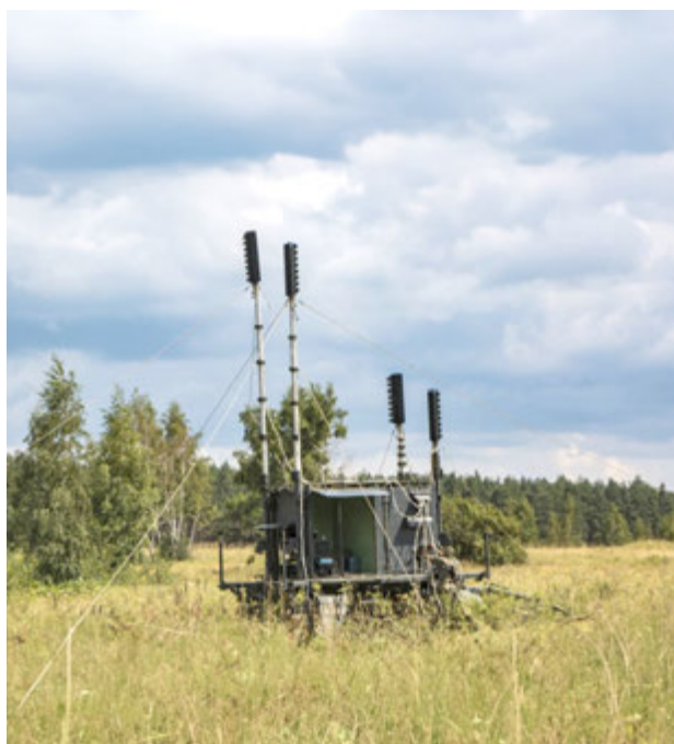
Figura 3: Jammer R-330Zh Zhitel.
